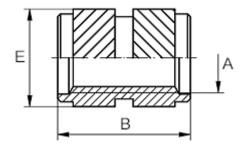
Female thread A = M10 Length B = 12.7 Min distance to edge = 5.5Outer diameter E = 12.5Recommended bore diameter W +0.1 = 11.9
